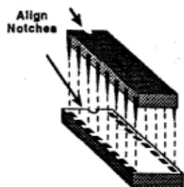
When inserting an IC into a socket, make sure that the pins are straight and the notches are aligned.
